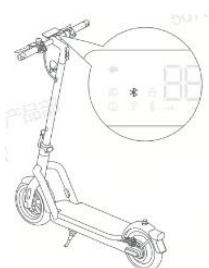
2. Power on the scooter, a blinking Bluetooth icon indicates the scooter is waiting to be connected.
