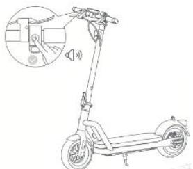
Note: For your safety, your new scooter cannot be fully activated before it is linked to your mobile phone; it will beep continuously after being turned on and its speed will be limited to 10 km/h. When the scooter is used for the first time, it must be activated via the NAVEE app, where you can follow a safety tutorial. After the scooter is activated, the beeping will stop and the speed restriction will be lifted.
